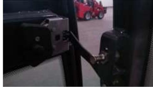
On opening, the cab doors automatically lock into the door lock. Release this lock to close the door.
