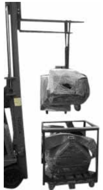
Lifting the feed hopper
