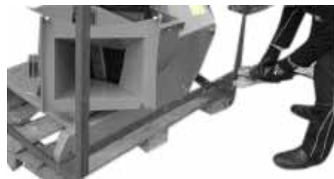
Remove the steel frame
