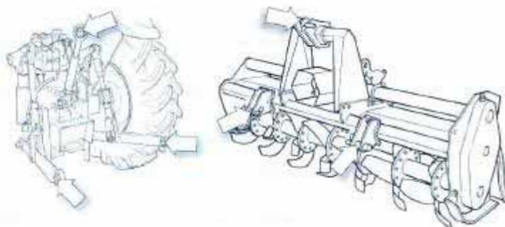
When this has been done, remove pins A from the machine and attach the lift arms of the tractor to the machine using these A pins. Next, attach the top rod of the tractor to the top coupling point of the machine.
