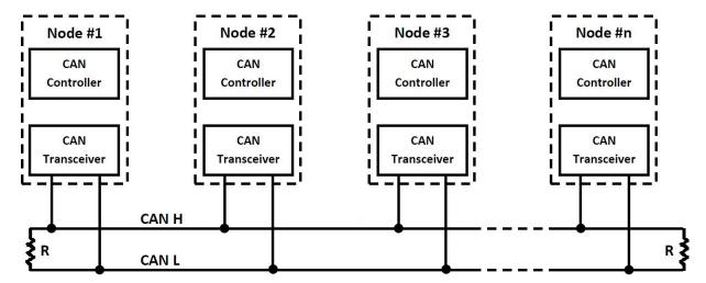
It's terminated at both ends with  $120\Omega$  resistors in order to adapt the lines to a fixed impedance, avoiding reflections or other problems that can occur at high frequency of CAN (from 125KBaud to 1Mb). Placing these resistors on a node should be avoided since the bus line loses termination if the node is disconnected from the bus.
