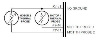
Thermal Probe Wiring
